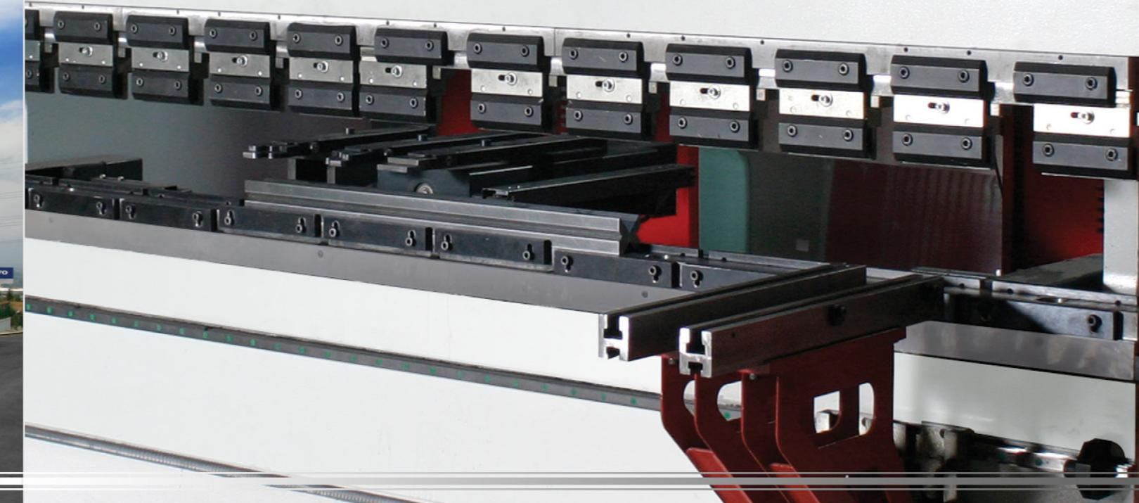
Our model year 2011 Baykal brand CNC press brake bending machine has 5-axes and it can bend the parts conically. Along with our bending machine, we have the most commonly used punches and die blocks in the sector which enable us to bend various thicknesses at various angles and can invest in new ones to meet our customers' needs. With its 160 ton capacity and 3100 millimeter working length we can meet the most demanded requests of the metal sector.
